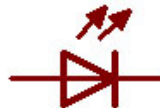
LED symbol, positive pin on the left, negative pin on the right
